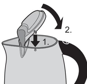
1. Put the lid onto the water kettle as shown in fig. (Fig. 2/1.).
