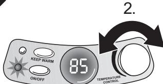
3. Now set the desired temperature by turning the control knob (Fig. 4/2.)
