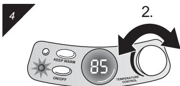
3. Now set the desired temperature by turning the control knob (Fig. 4/2.).
