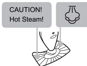
Fig. 1: Steam warning notice on steam base
