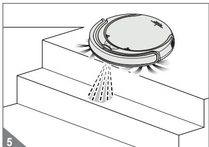
With the aid of 3 fall sensors, your robot vacuum automatically detects drop-offs in front of it (Fig. 5). If a drop-off is detected it changes its direction of travel and continues to clean in the opposite direction.
