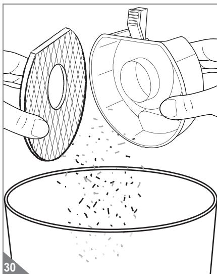
5. Hold the dirt bin over a dustbin with the filter inserted.
